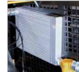
The compressed air is cooled to 7 °C above ambient temperature. Accumulated condensate is able to drain away easily, as the compressed air cooler is installed at an angle, whilst the hot exhaust gasses from the motor are also used to aid condensate evaporation. This design consequently ensures reliable frost prevention during the winter months.
